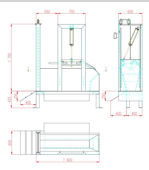
Stunning holder for pork is used for pig's stunning at the slaughterhouses. The holder is delivered in length of 1600 mm in right or left design. The entering falling gate is controlled by hand. The gate's weight is compensated by counterweight. Tipping side is used for coming out of the stunned pig from the holder and is pneumatic operated. Surface finishing is hot-dip galvanizing, according to the customer's wish can be delivered in stainless steel.
